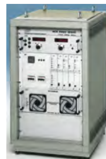
Design Example HCK 5000 - 12500 12,5kV / 800mA
